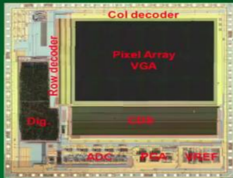
CMOS Active Pixel Sensor With Intra-Pixel Charge Transfer Camera-on-a-chip
